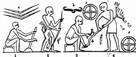
Ancient Egyptian Chariot-makers. Fig. 1, Sawing out the Axle; 2, Preparing the bent pieces of Wood, a, b; 3, 4, Shaping the Pole, d; c, e, Wheels.
